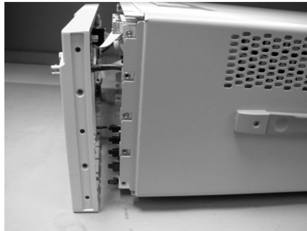
Figure 4-33. Slide Front Panel Away From Mainframe
