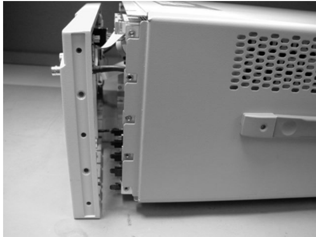
Figure 4-8. Sliding Front Panel Away From Mainframe
