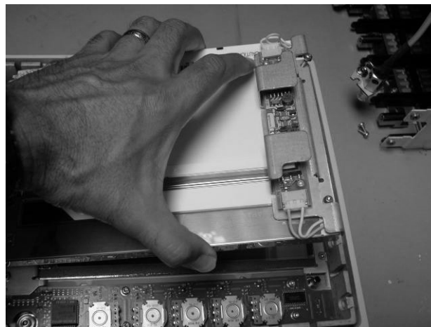
Figure 4-17. Removing the Display
