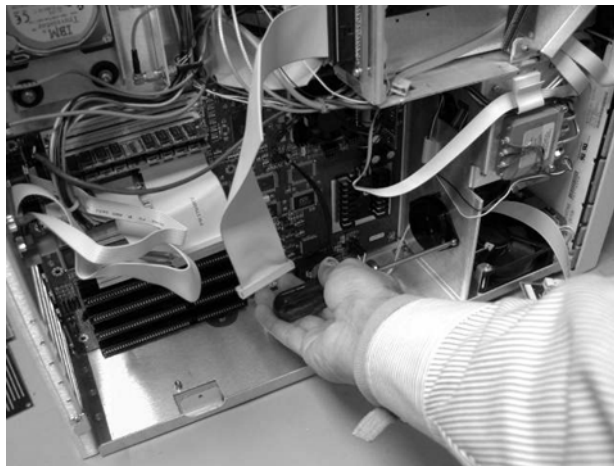
Figure 4-38. Removing the Speaker Screw
