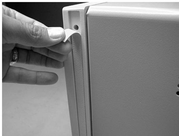
Figure 4-6. Removing the Trim Strips
