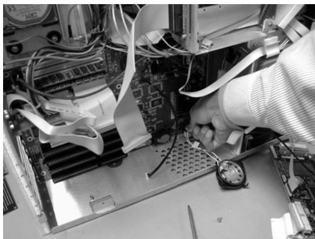
Figure 4-39. Disconnecting the Speaker Cable
