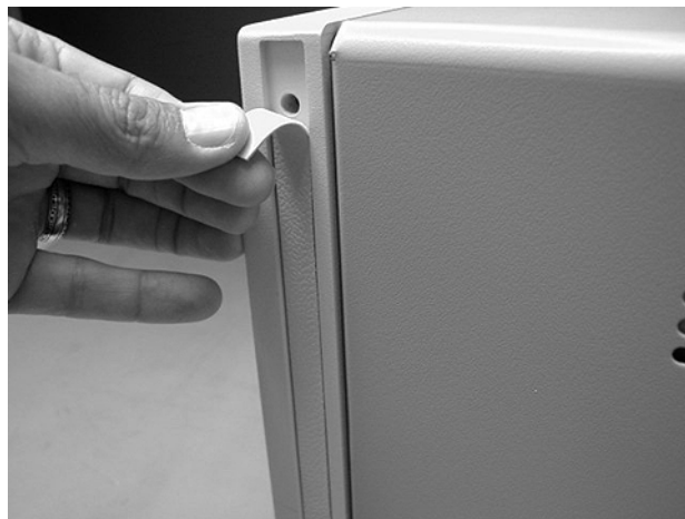
Figure 4-26. Removing the Trim Strips
