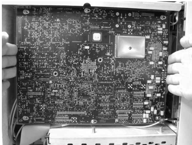
Figure 4-50. Sliding the Board to the Right
