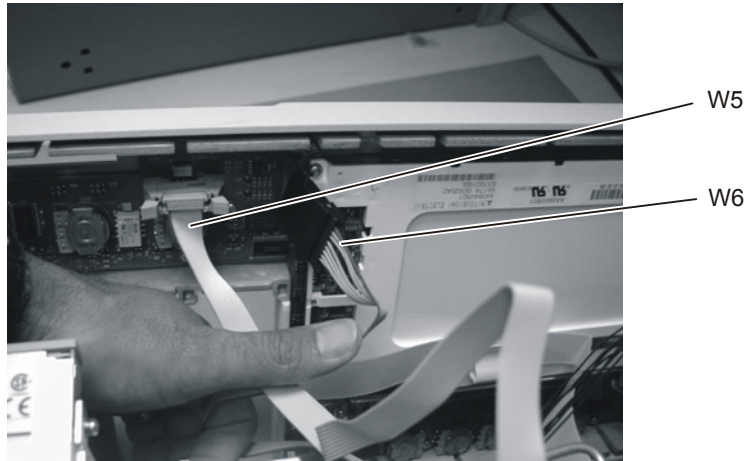
Figure 4-10. Removing the W5 and W6 Ribbon Cables
