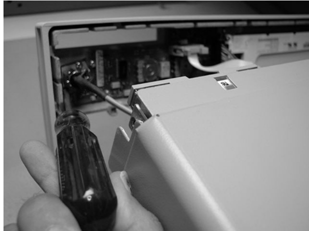
Figure 4-9. Removing Screws that Secure the Cal Connector
