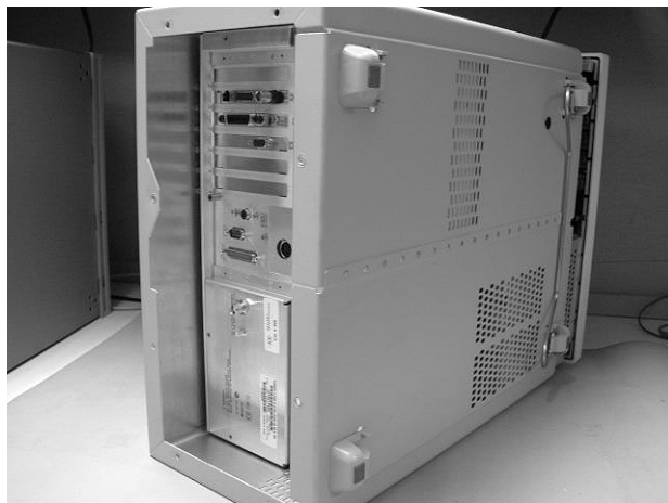
Figure 4-5. Sliding Cover off Mainframe
