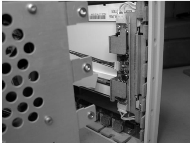
Figure 4-28. Accessing the Inverter Board
