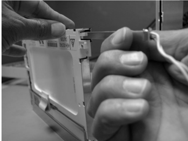
Figure 4-20. Removing the Backlight
